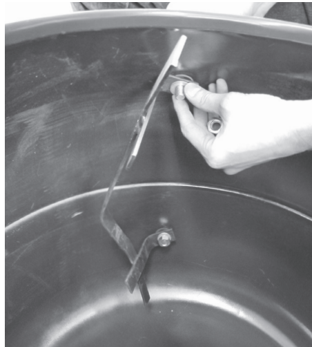
Install paddles with short side facing outward, towards top of the drum.
