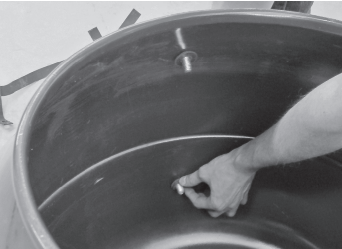
Place rubber washers onto bolts.
