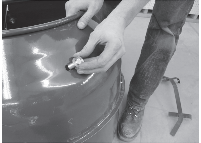
Insert bolts through drum.
