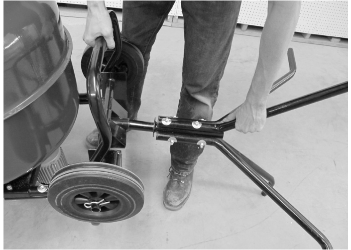
Lift mixer slightly and insert pedestal.
